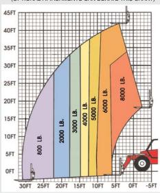
Capacities shown in pounds/feet are the maximum recommended load limits at the indicated extensions of the boom. Capacity ratings are based on a 48" homogeneous cube and are in accordance with ANSI/ASME B56.6 stability standards. Capacity reductions must be made for extended load centers and when used with various other attachments, contact MANITOU NORTH AMERICA, INC.
